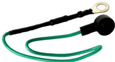
232761 Resistor Servicing: 27SI/200 150 Ohm resistor. Resistor connects from battery terminal to pin-type R-terminal for faster 'cut-in' speed.
