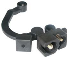
234110 Terminal Block Servicing: A3TA6491, A3TA6491A, a3tb0891, A3TB0891A, a3tb0891b, A3TB0891C ID/ mount. hole 6.50, Length 137.00, Height 28.70 B+ M8. D+ M5.
