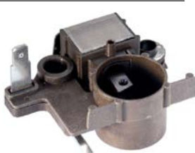
134754 Regulator Replacing: a866x07470 Servicing: A5T31772, A5T31773, A5T31774 14 V, 14.6 V setting, Dist. mount. holes 40.00, Terminal type I
