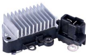
133872 Regulator Replacing: MD604751 14 V, 14.6 V setting, Dist. mount. holes 57.50, Terminal type IG-L Repair circuit: Cargo 133259. The L-terminal does not drive the choke.
