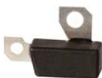
233119 Condenser Replacing: 1988972 Servicing: 17SI, 21SI, 33SI, 34SI, 10479864, 10479868, 10479870, 10479915, 1101215, 1101252, 1101258, 1101290, 1105585, 1105613 Length 38.50, Height 13.30, Width 25.55 1.50 µf capacitor.
