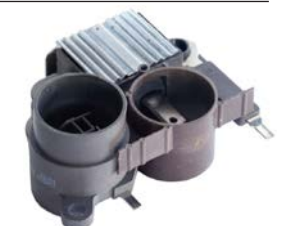
135033 Regulator Replacing: a866x15072, a866x13571, a866x13471, a866x11872, a866x11870 Servicing: A1T02091, A1T02191, a1t03191, A1T03191ZC, A1T03195ZC, A1T04491, A1T04495, A1T04691, A1T04791, A7T00171, A7T00191 14 V, 14.6 V setting, Dist. mount. holes 47.00, Terminal type D-IG-L
