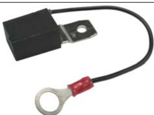
139387 Condenser Replacing: 6270-369a Servicing: AC203 Length 45.25, Width 16.65 3 \mu F-110 V.
